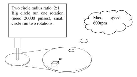
Electronic gear ratio is 131072:5000 or pulses per rotation is 5000, PLC max output pulse frequency is 200KHz.
