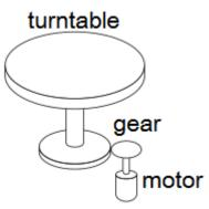
Because it can only rotate in one direction, after a certain period of time, the number of revolving cycles will always exceed the upper limit of absolute value encoder.
