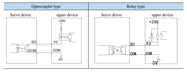
Note: The maximum load current is 400 mA (if the brake motor is controlled by SOx, please confirm the brake current first, and if it is larger than 400 mA, please use the intermediate relay).
