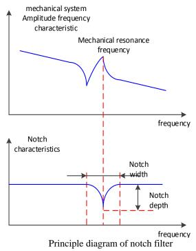
The servo driver has five sets of notch filters, each with three parameters, notch frequency, notch attenuation and notch bandwidth. The first and second notches are set automatically, and the third, fourth and fifth are set manually.
