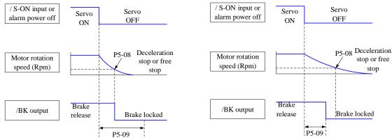
Since the brake of the servo motor is designed to be used as a position holder, it must be activated at the right time when the motor stops. While observing the action of the machine, adjust the user's parameters.
