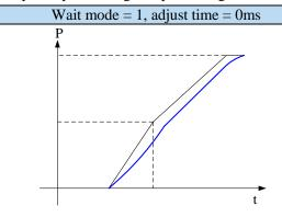
After the drive output 1-segment position command, it will not wait for the completion of motor positioning, and start the next position command at once.
