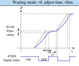
After the drive output 1-segment position command, it will wait for the completion of motor positioning, and pass the adjust time, then start the next position command. T1 is positioning time, t2 is adjust time. Refer to parameter P4-11.
