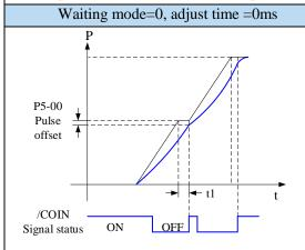
After the drive output 1-segment position command, it will wait for the completion of motor positioning, and then start the next position command at once. T1 is positioning time, which means the time from pulse output complete to the output of positioning completion signal.
