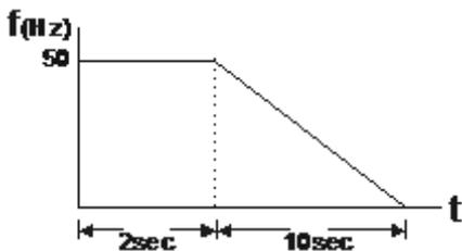
Therefore the distance travelled by the motor after the stop command is given = number of rounds x circumference =  $175 \times 2\pi r$ . That means the turbttable went back to the top after 175 rounds.
