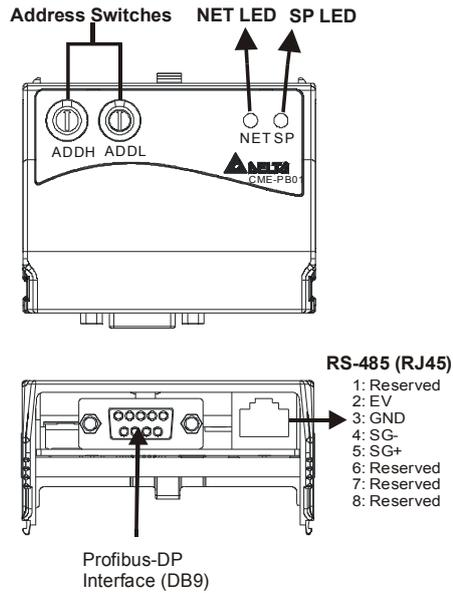
1. SP LED: Indicating the connection status between VFD-EL and CME-PD01.
