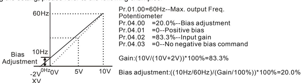
**Example 4: Use of 0-5V potentiometer range via gain adjustment**
