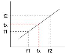
$$t_x = t_2 - \left( \frac{f_2 - f_x}{f_2 - f_1} \right) \times (t_2 - t_1) = t_2 - \left( \frac{f_2 - f_x}{10} \right) \times (t_2 - t_1)$$
