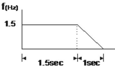
Therefore the distance travelled by the motor after the stop command is given = number of rounds x circumference =  $1.5 \times 2\pi r$ . That means the turbttable stopped after 1.5 rounds.
