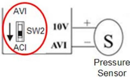
Wiring of the pressure sensor:
