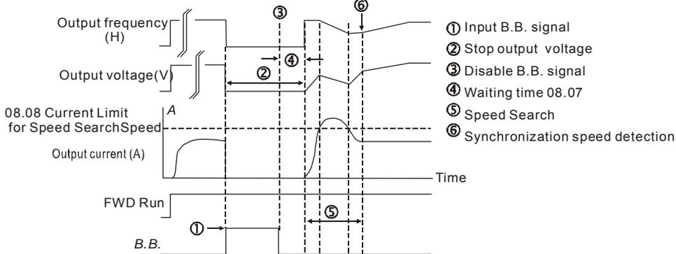
Fig 1: B.B. Speed Search with Last Output Frequency Downward Timing Chart (Speed Search Current Attains Speed Search Level)
