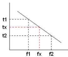
$$t_x = t_1 + \left( \frac{f_2 - f_1}{f_2 - f_x} \right) \times (t_2 - t_1) = t_1 + \left( \frac{f_x - f_1}{f_2 - f_1} \right) \times (t_2 - t_1)$$
