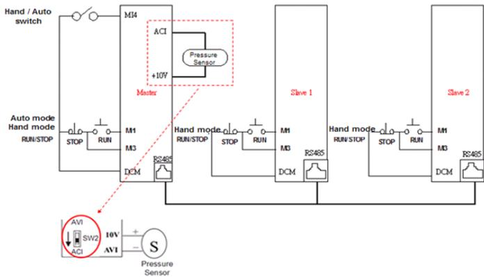
Wiring of the pressure sensor:
