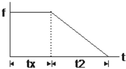
$$S = n \times \left( \frac{t_x + (t_x + t_2)}{2} \right)$$
