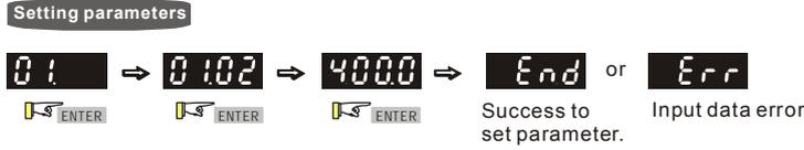
NOTE :In the parameter setting mode, you can press to return the selecting mode.
