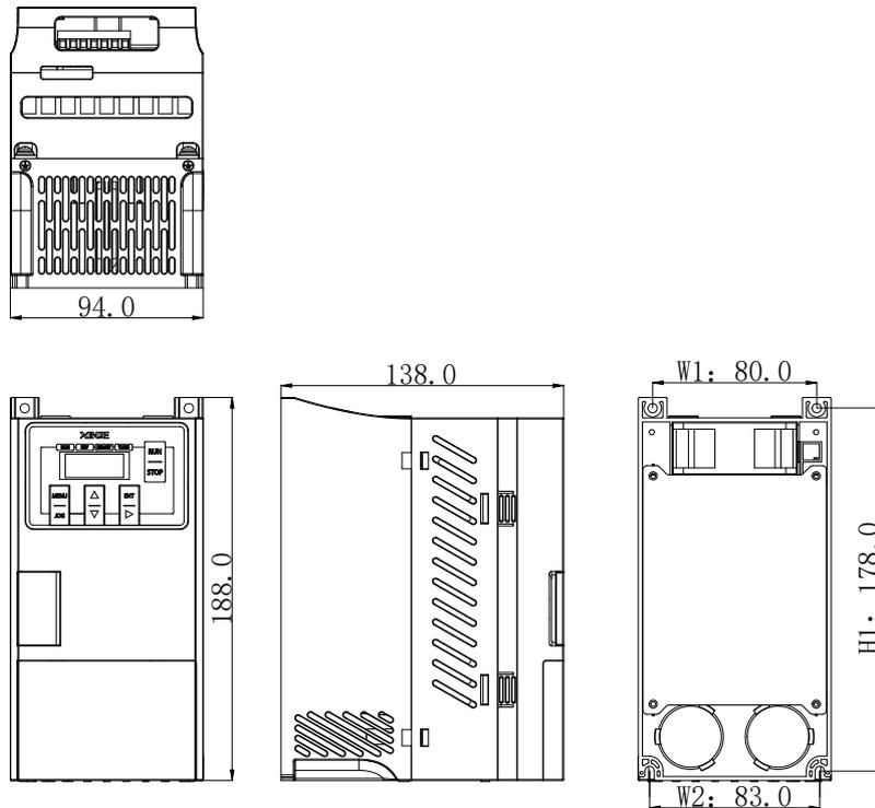
Note: the installation screw is M4.
