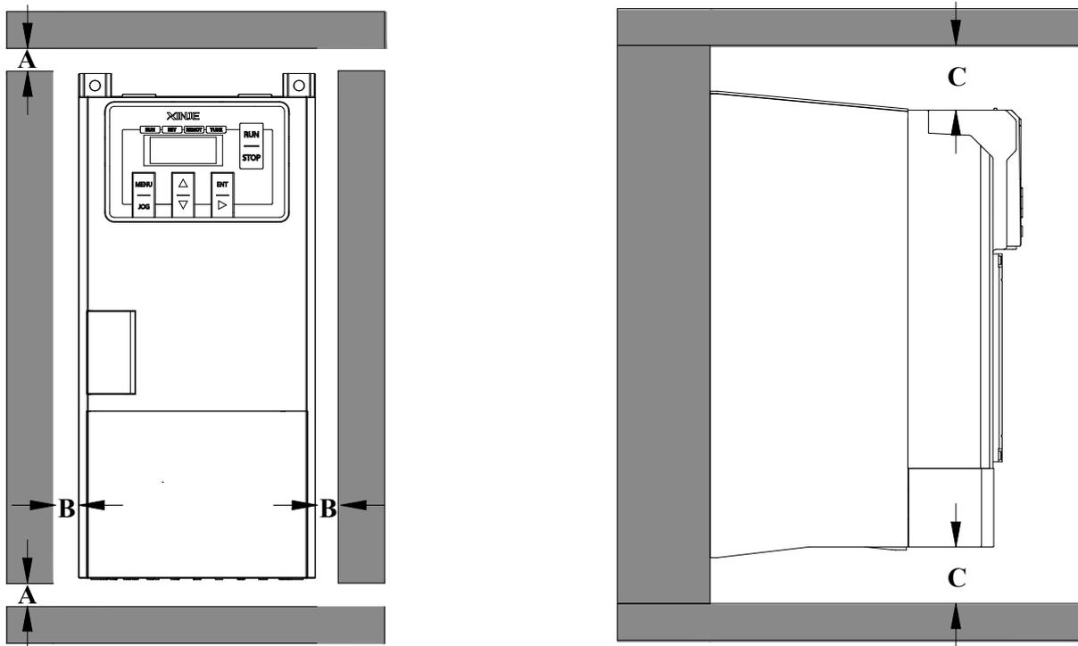
Note: the distance of A and B is more than 50 mm, and the distance of C is more than 100 mm.
