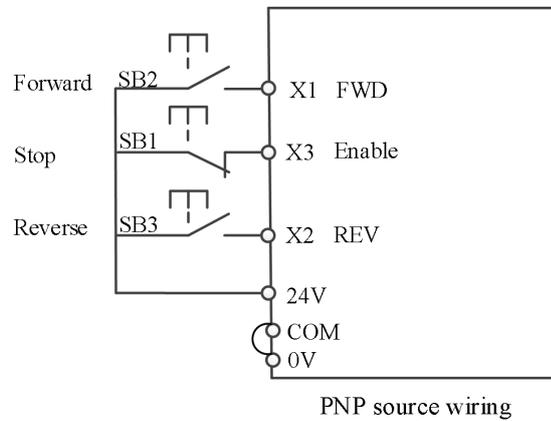
As shown in the figure, in the control mode, when SB1 button is closed, press SB2 button, the frequency converter rotates forward, and then press SB3 button, the frequency converter reverses, SB1 button is disconnected, and the frequency converter stops. During normal start-up and operation, SB1 button must be kept closed, SB2 and SB3 button commands will take effect at the closing action edge, and the operation state of frequency converter is subject to the last action of the three buttons.
