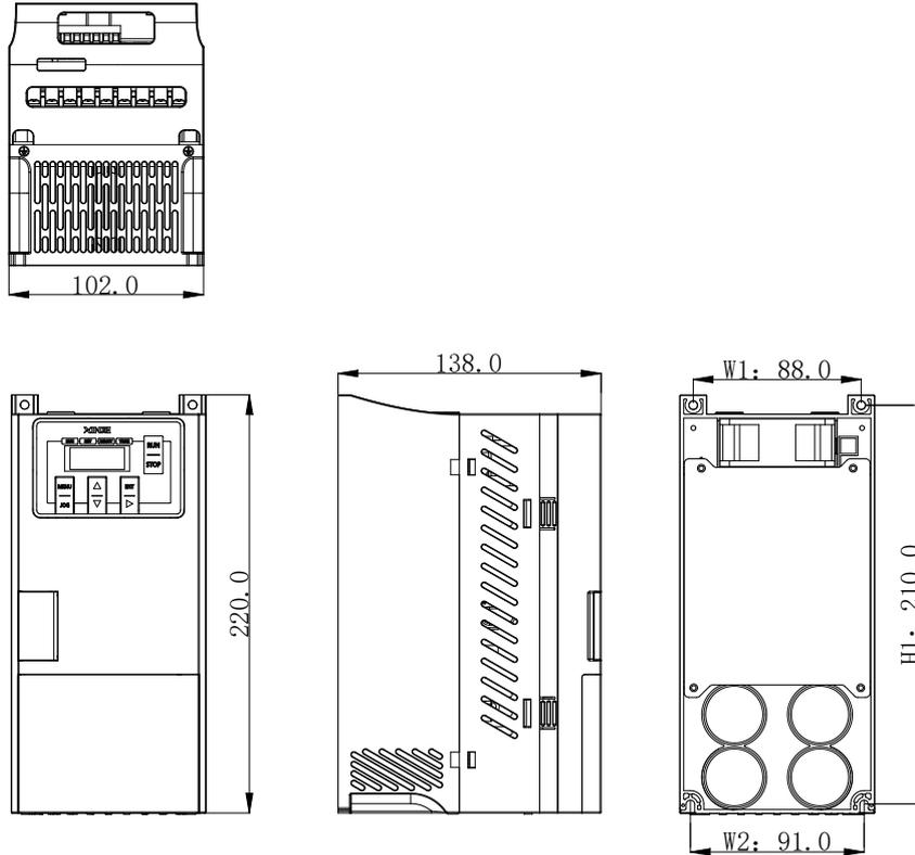
Note: the installation screw is M4.
