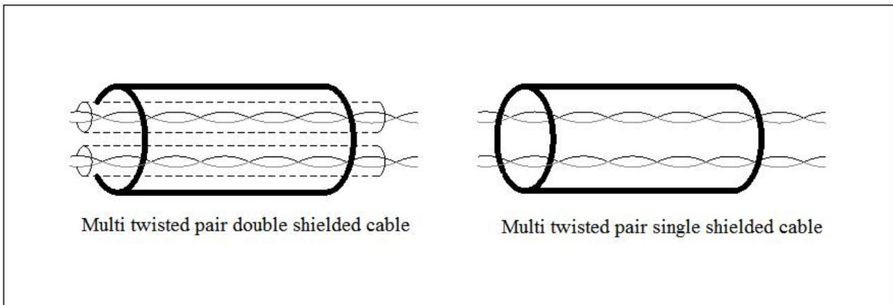
Relay cables need to be shielded with metal braid.
