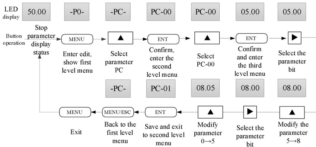
In the three-level menu, if the parameter has no flashing bit, it means that the parameter cannot be modified. The possible reasons are as follows:
