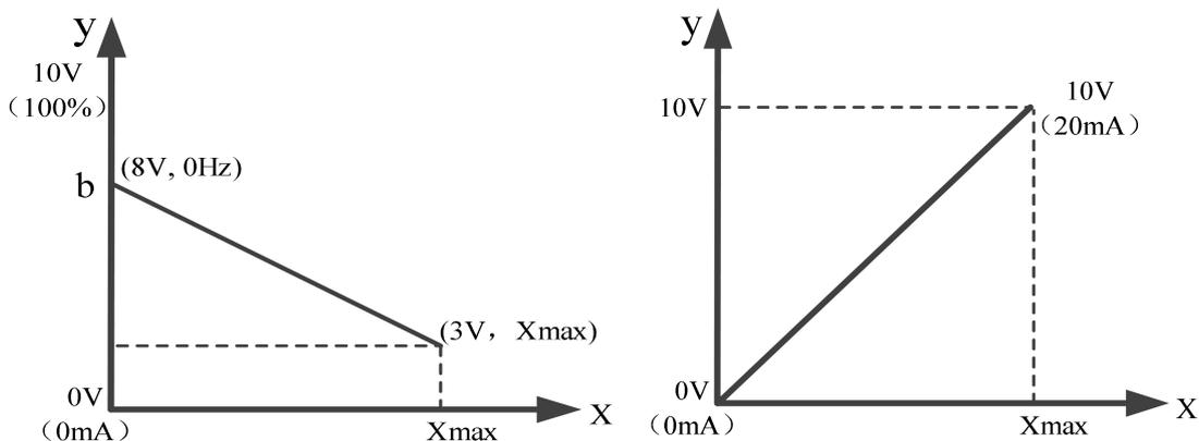
$$\text{Zero bias coefficient} = \frac{\text{output at 0Hz}}{\text{max output}} \times 100\%$$
