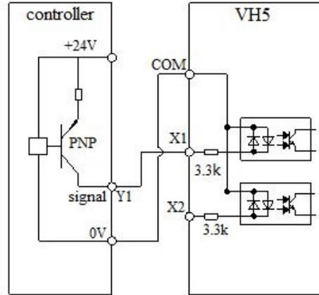
Single VFD uses internal 24V source wiring
