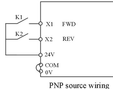
As shown in the figure, in this control mode, when K1 is closed, the converter runs in forward direction. When K2 is closed, the inverter runs in reverse. When K1 and K2 are closed or disconnected at the same time, the inverter stops running.
