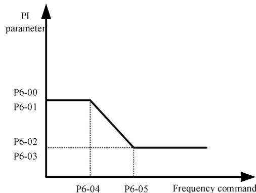
By setting the proportional coefficient and integral time of the speed regulator, the speed dynamic response characteristics of the vector control can be adjusted.
