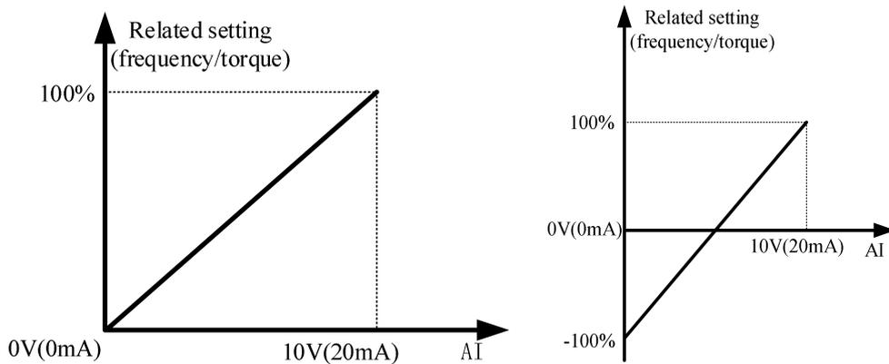
The functions of AI curve 1 (P2-18~P2-21) /AI curve 3 (P2-26~P2-29) are same to AI curve2.
