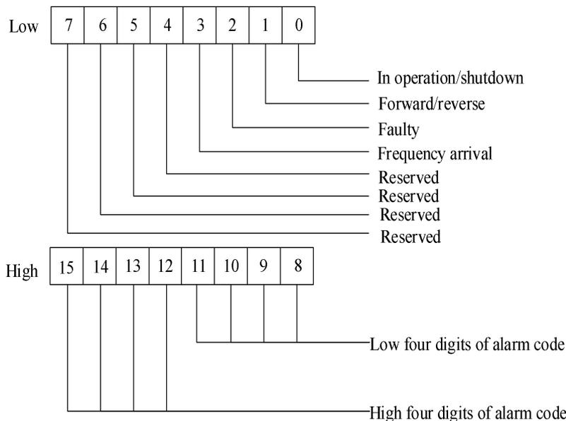
For example: U0-69=H.2C04, hexadecimal 2C converted to decimal is 44, which means that the current fault code is Err44, hexadecimal 04 converted to binary is 100, which means that it is in a fault state.
