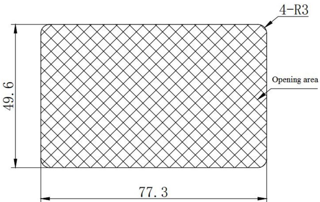
**Installation instructions:** according to the dimensions in the figure above, open the hole on the outer surface of
