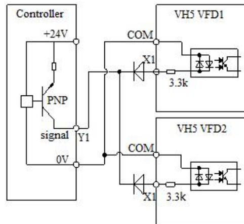
Multi-inverter uses internal 24V source wiring
