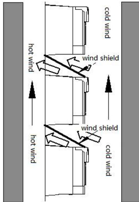
Note: when installing vertically, the wind shield must be added, otherwise it will cause mutual influence between multiple inverters, resulting in poor heat dissipation.
