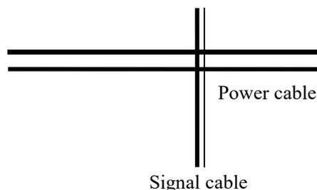
6. Weak current grounding wires such as control signals and sensors must be grounded independently from strong current grounding wires.
