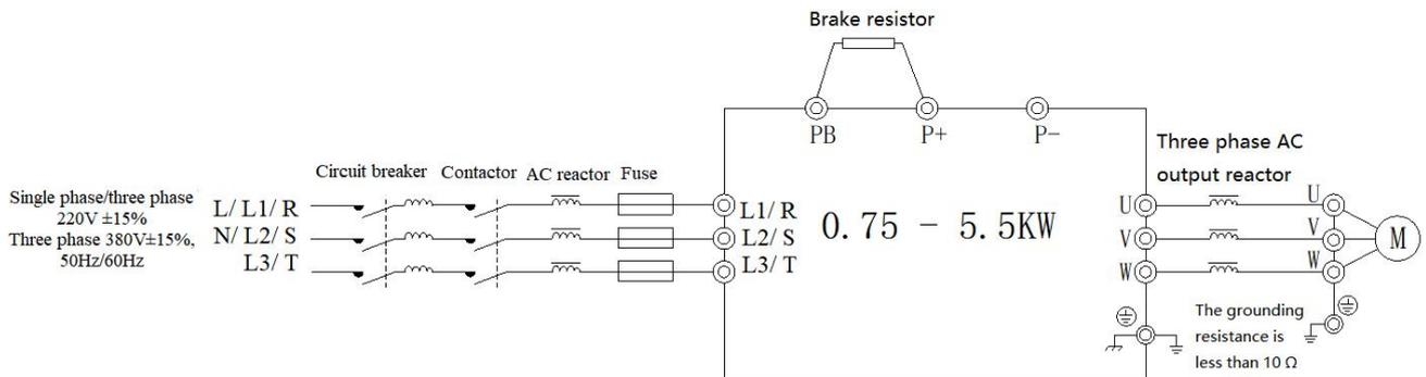
Note: circuit breaker, contactor, AC reactor, fuse, brake resistor and output reactor are optional parts. Please refer to chapter 6 for details.
