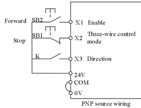
As shown in the figure, in the SB1 button closed state, press the SB2 button, the frequency converter runs, K opens the frequency converter forward, K closes the frequency converter reverse; When SB1 button is off, the inverter stops. During normal start-up and operation, SB1 button must be kept closed, and SB2 button command will take effect at the closing action edge.
