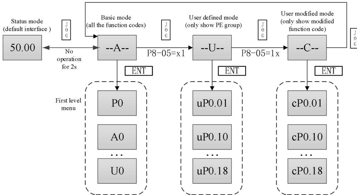
P8-05 is used to control the display of user defined group and user modified group parameters.
