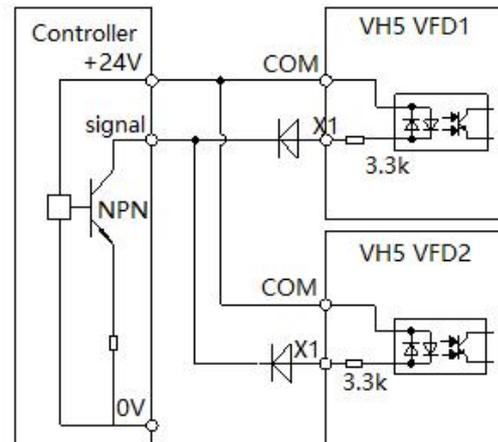
Multi-inverter uses external 24V leakage wiring
