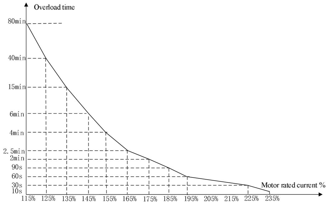
(1) Theoretically, when the running current of the motor reaches 175% times of the rated current of the motor, the motor overload (Err10) will be reported after continuous running for 2 minutes; When the running current of the motor reaches 115% of the rated current of the motor, the motor overload (Err10) will be reported after continuous operation for 80 minutes.
