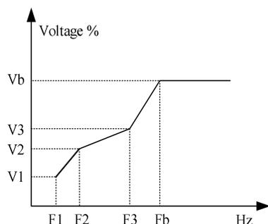
Note: V1 ~ V3: voltage percentage of section 1 ~ 3 of multipoint VF curve. F1 ~ F3: frequency point of section 1 ~ 3 of multipoint VF curve.
