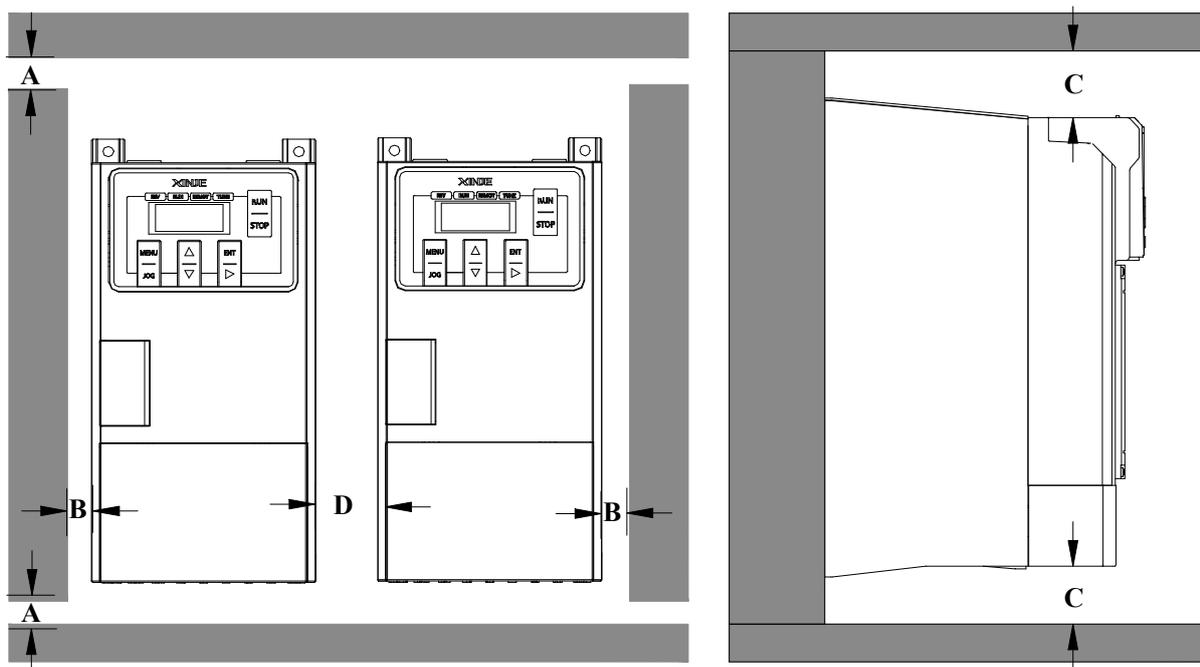
Note: the distance of A and B is more than 50mm, and the distance of C and D is more than 100mm.
