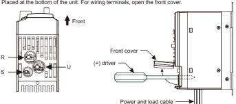
Open the front cover, there are the rotary switch, DIP switch, power input part
