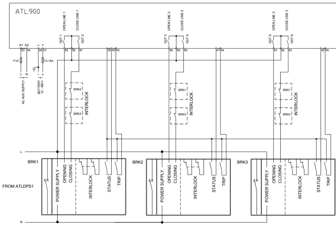
Example of power line connection + breakers + tie breakers
