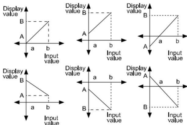
Display scale function is able to change display value for max./min. measured input by setting high-limit scale [ Hi Scale ] and low-limit scale [ Lo Scale ].
