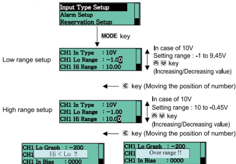
When High / Low graph setup with wrong value and pressing **MODE** key for save, error message is indicated as above.
