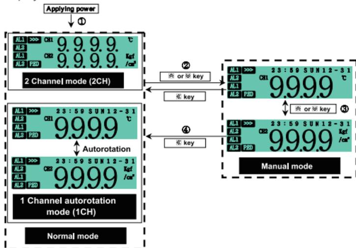
If applying power, it will be indicated by mode setup (2CH or 1CH) on display mode parameter.
