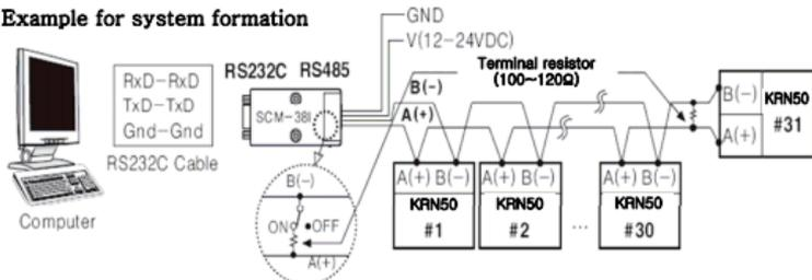
It is recommended to use Autonics communication converter SCM-381(RS232C to RS485 converter), SCM-US481(USB to RS485 converter).
