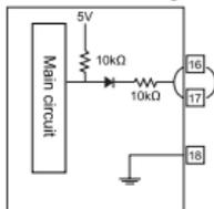
**(16) Recording start/stop when power on [PWR On State]**
