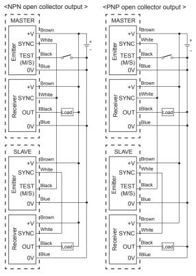
\*\*Connect 'TEST (M/S)' of SLAVE emitter to 'SYNC' of MASTER.
