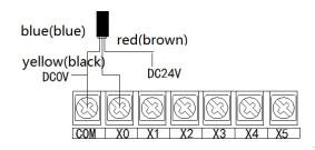
Three wires (NPN) proximity switch wiring example
