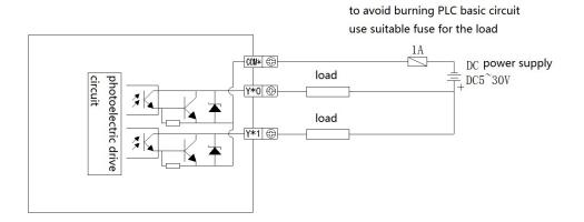
Below is wiring of T type integrated PLC&HMI and servo drive
