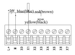
Three wires proximity (NPN) switch wiring
