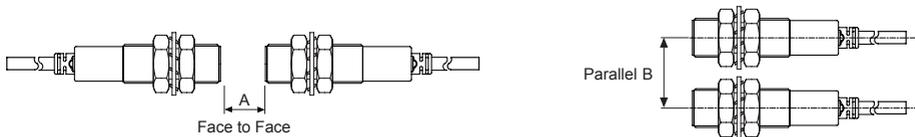
When sensors are mounted on metallic panel, it is required to protect the sensors from being affected by any metallic object except target. Therefore, be sure to provide a minimum distance as below chart indicates.
